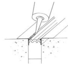
**IMPORTANT:** Polysulfide left between the wrinkles of the bellows could constrain movement – using a caulk knife, remove excess sealant and blend what remains into the bellows.
