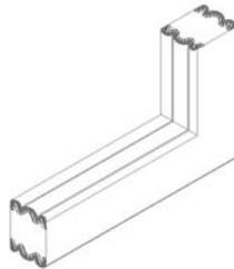
Connect straight run material to in-place terminations and transitions (see step #8). Cut closing pieces 3/8-inch (10mm) longer than the opening to be joined. Compress material longitudinally to fit.
