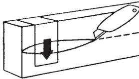
**IMPORTANT:** Work quickly and deliberately after cutting the shrink-wrap to avoid material expanding beyond a usable size.
