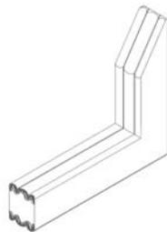
Connect straight run material to in-place terminations and transitions (see step #8). Cut closing pieces 3/8-inch (10mm) longer than the opening to be joined. Compress material longitudinally to fit. The factory-sealed end acts as the termination and points up or down to best block or direct water flow.
