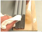
To remove the factory-applied release agent, thoroughly wipe the cured silicone face, tops and grooves of the bellows next to the face, and along the sides with a lintfree rag made damp with water.
