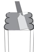
**IMPORTANT:** All sticks of WFR3 foam MUST have a coating of intumescent on the faces of all joints. This ensures that joints do not compromise the fire barrier.
