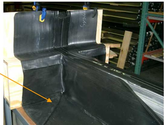
NOTE: It is difficult to accurately represent all substrate contours that the side-sheets will come in contact with. For this reason factory-welded side sheets cannot be guaranteed to fit and may require field modification by the contractor.
