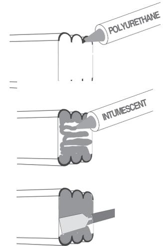
**IMPORTANT:** All sticks of SSF2 foam MUST have a coating of intumescent on the faces of all joins. This ensures that joins do not compromise the fire barrier.
