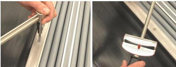
**IMPORTANT:** If you strip or cross-thread a screw while installing it, remove the screw and use a 6mm tap and to manually re-thread the hole. Reinstall the nylon washer and screw.
