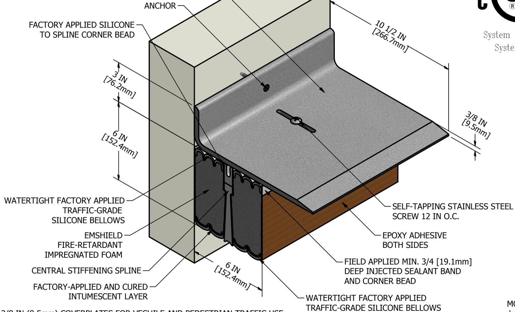
NOTE: 3/8 IN (9.5mm) COVERPLATES FOR VEHICLE AND PEDESTRIAN-TRAFFIC USE
